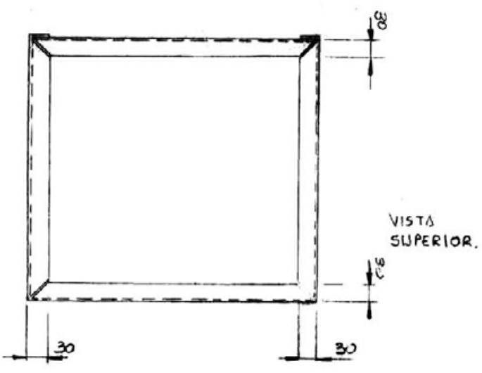
Dimensions of the base with format of 19'' rack. Preferably in steel plate of 1 mm. Also can be made in wood and Formica with aluminum edges. If a rack space is not needed, the front can be replaced by a door and used to hide the CPU from up to two PCs
