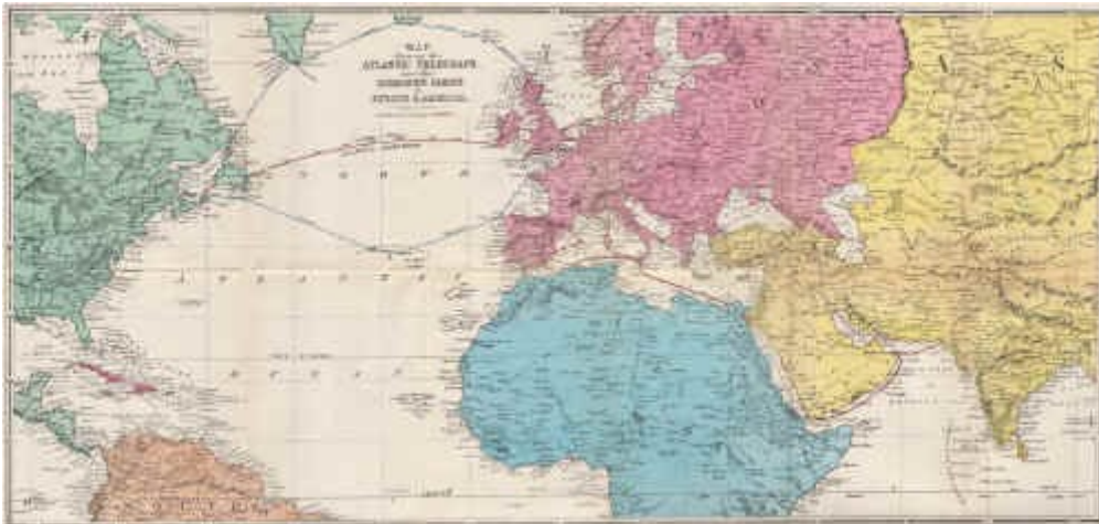
1865: Map Shewing the Atlantic Telegraph and other Submarine Cables in Europe and America from The Atlantic Telegraph . Note also the route of Tal Shaffner's proposed northern cable.
